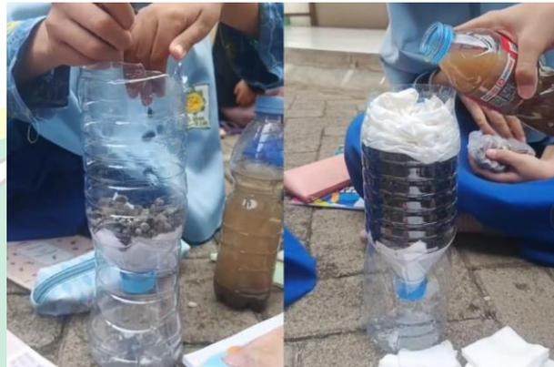
**Gambar 4. 6 Percobaan Filter Air**
