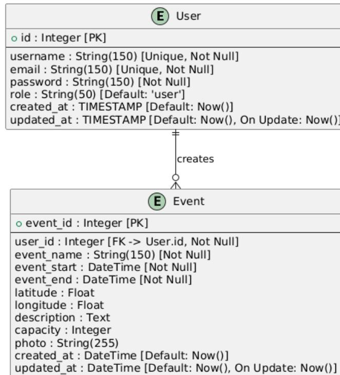
Gambar 4. Entity relationship diagram database
