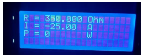
Figure 3. Data display of electrical resistance, electric current, and output electric power on LCD screen
