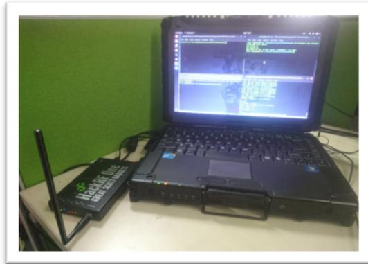
Gambar 6. Simulasi ADS-B Transponder
