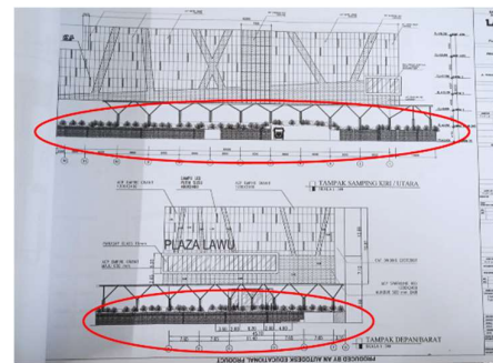
Gambar 19: Tampak Lokasi Vertical Garden di Fasad Bangunan Sumber: Tim Manager Building Plaza Lawu Madiun, 2020
