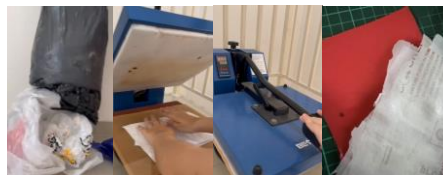
Plastic waste collection > heat press preparation > heating process > fused plastic
