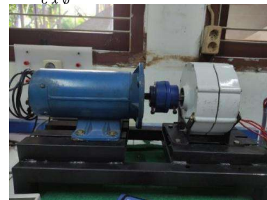
Gambar. 4 DC Motor 180V DC Magnet Permanent
