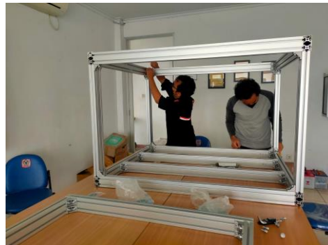
Figure 4. Fabrication of Prototype of Housing 3D Printer
