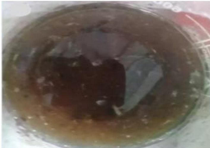
Figure 3.7. Lab made acacia-frankincense bio resin
