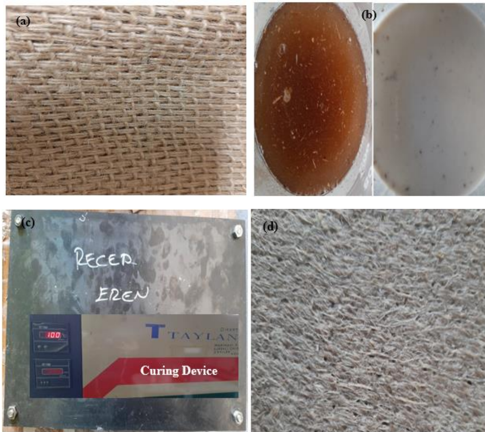
Figure 3.9. a) Enset fabric b) Acacia and frankincense gum bio resin c) Used hand layup set 20 and curing device d) Enset fabric reinforced green composite material
