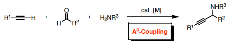
Scheme 40. General metal-catalyzed \text{A}^3 -coupling reaction.
